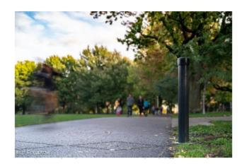
The MULTI system uses the electromagnetic ZELT inductive loops in the pavement to detect bicyclists and the infrared PYRO sensor in a post to detect pedestrians and direction of travel of all users.
