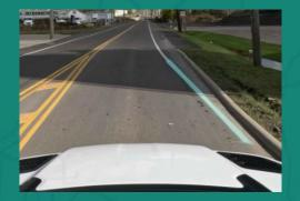
1800+ miles pavement striping detected, classified, and condition rated
