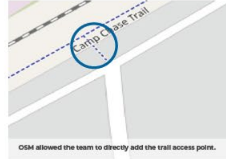
OSM failed to use the Camp Chase Trail for routing due to a missing trail access point.
